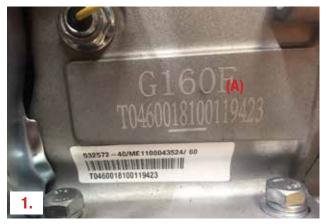
How Do I Find a Loncin Engine Model Number? What am I looking for? The Engine Model Number is scribed into the side of the alloy engine block. In the example "G160F"(A) in large font is the model number and that is what you need to look up parts.
