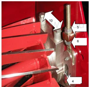
**CUTTER** - To adjust the cutter setting, slacken cutter hanger clamp bolts (4) at each side of the machine, and proceed as follows:
