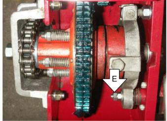
**CLUTCH** - To be certain that the clutch is fully engaged without possibility of slip, there should be approx. 1 1/2" of free movement (at the clutch operating lever knob) before the resistance of clutch operation is felt. This adjustment is made by means of the self-locking nut "E".
