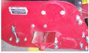
**REVERSING CUTTER** - A feature of this machine is that the cylinder may be easily removed, reversed end for end and replaced. This provides a new keen cutting edge. If the bottom blade is badly worn, this should be replaced at the same time that the cutting cylinder is reversed or replaced.
