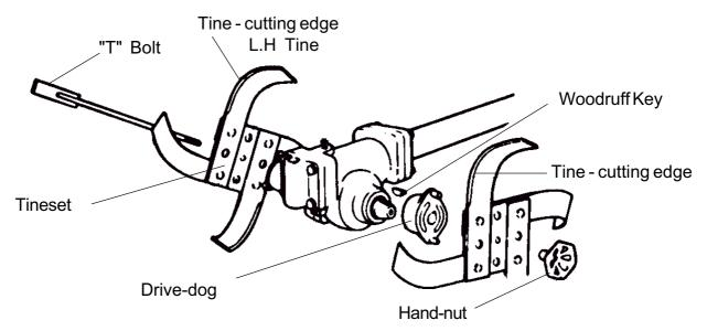
NOTE: To determine right or left hand tine - hold tine in horozontal position with cutting edge uppermost and pointing away from you.
